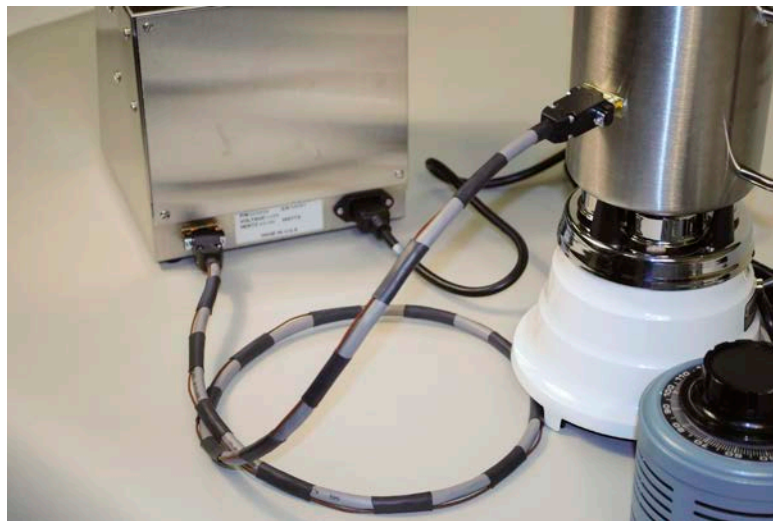
Figure 5-1 Cable Assembly Connected to Mixing Container
