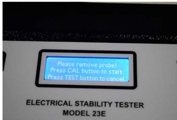
**Figure 6-2 Self Calibration Mode**
