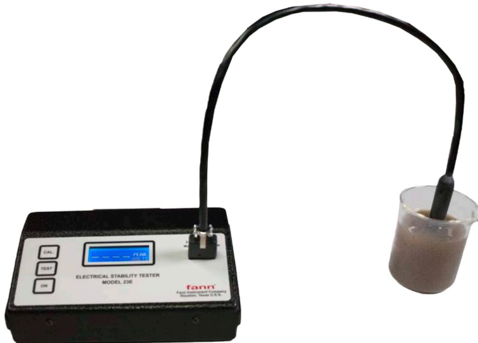
Figure 5-2 EST Probe immersed in sample
