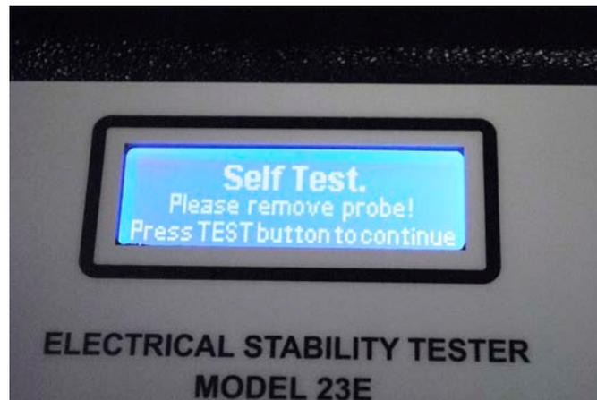
Figure 5-1 Self Test Mode
